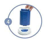
Slide your Inogen One Battery onto the charger with the handle of the battery up. The battery will only fit one way, and easily plugs into place as shown.
